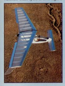
right at the 63-mph (55-knot) limit. The airplane is powered by a 25-hp, singlecylinder Rotax engine. At cruise settings the engine burns 1.7 gph.
